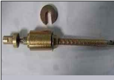
Swing arm NRB extractor & fitment tool Part No. : 37 0044 73 Application : For extracting & fitment of NRB
