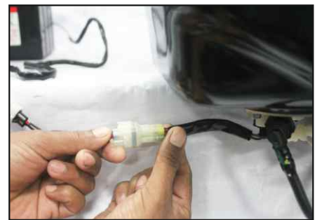
Pigtail 4 Pole to 2 Pole converter : Part No. : 37 2040 35 Application : For connecting fuel pump delivery checking unit to fuel pump.
