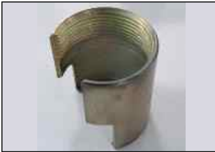
Bearing Race Extractor Part No. : 37 0044 78 Application : To Pull out steering race from fork Under Holder Bracket.
