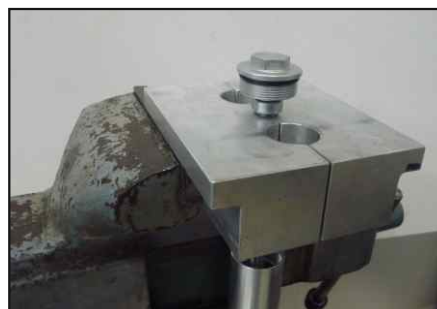
Fork clamping Block (Fork dia. 33mm)
