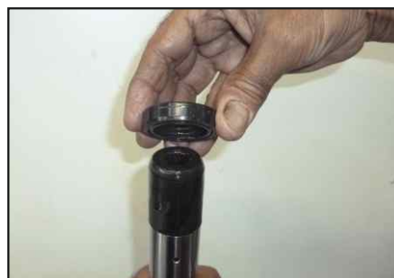
Oil seal protector tool (Fork dia. 33mm)
