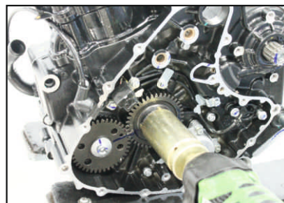
Balancer Lock Nut Tightening / Removing Tool
