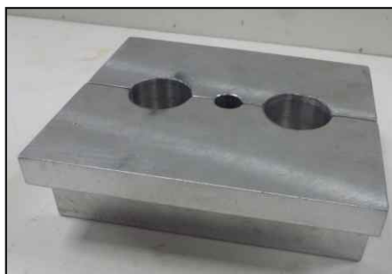
Fork clamping Block (Fork dia. 33mm)
