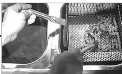
2nd Stage: Clean with Diesel + oil 1:1
