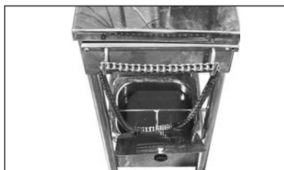
Final Stage : Hook chain for dripping of excess oil
