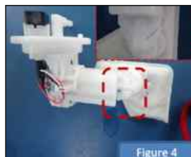
Check the gap between the Casing & Filter material
