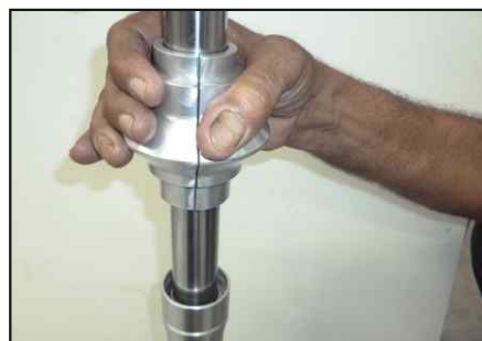
Oil seal & Guide bush fitment tool (Fork dia. 33mm)
