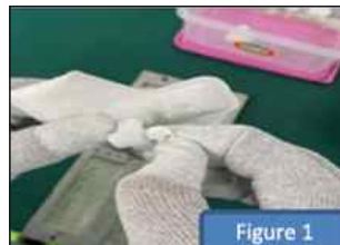
Remove the Dust cap from the filter
