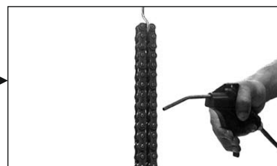
Blow Low Pressure Compressed Air
