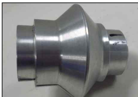
Oil seal & Guide bush fitment tool (Fork dia. 33mm)
